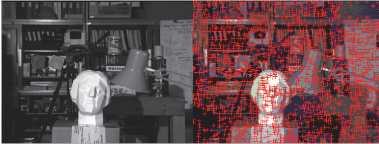
Figure 8. Edge detections in a features-based algorithm.
