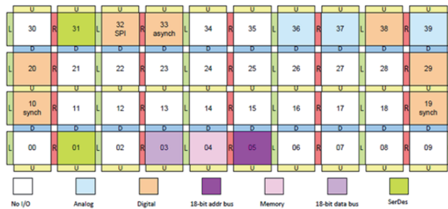
Figure 1. Block diagram of SEAForth 40C18, showing I/O and direction ports [16].
